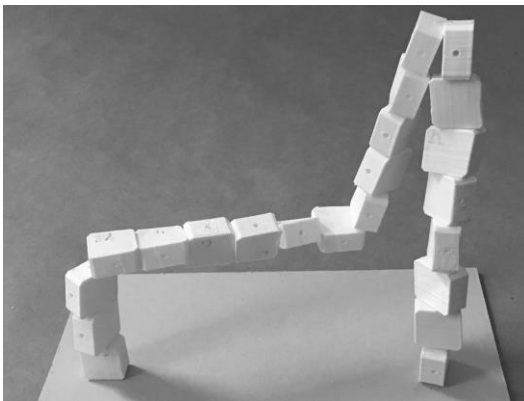
Figure 23. A simple, indeterminate arch exhibiting multiple stable states (a-c) which appear more or less frequently in accordance with how they minimize a function of the kink angles. (d) shows a closeup of a kink.
