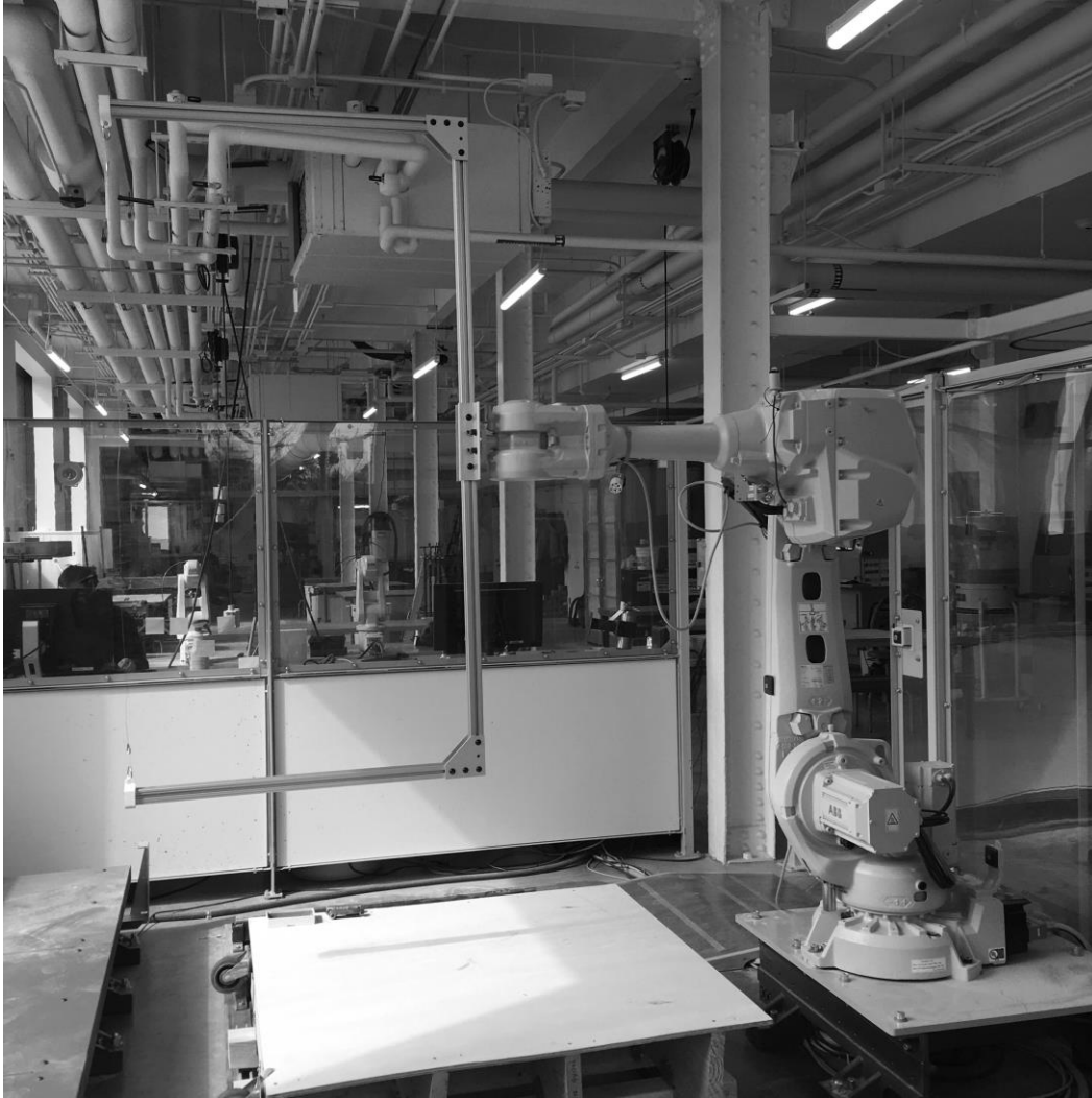
Figure 27. ABB IRB 4600 6-axis robotic arm at Cornell AAP Rand Hall fabrication lab, with custom 6' hot wire cutter end effector mounted to flange.
