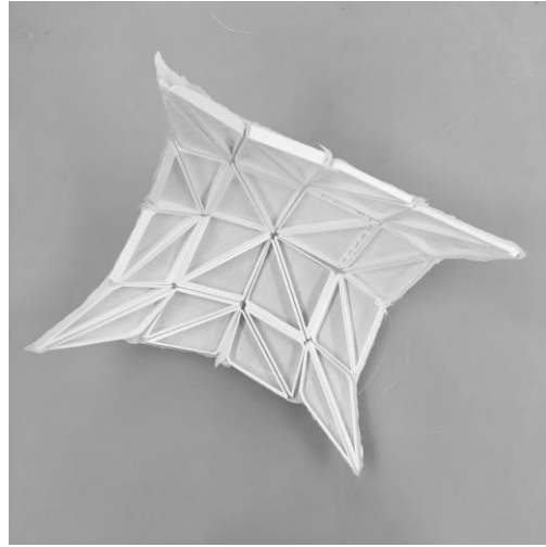
Figure 26. Triangulated shell model, composed of rigid triangular frames. Tensioned by nylon cord sewn through attached fabric along the periphery.
