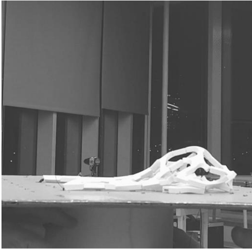
Figure 24. Initial dome prototype, (left) before, and (right) after tensioning cord
